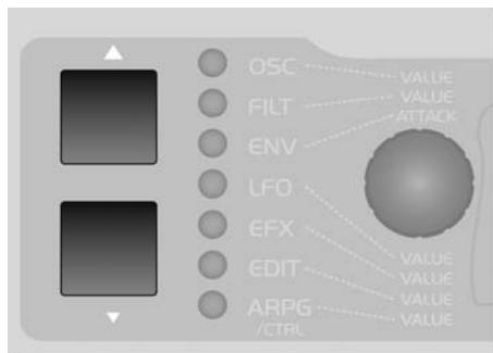
Rotate the ATTACK encoder while you repeatedly engage a key to hear the note. The further you turn the encoder up, the longer it takes for the sound to achieve maximum volume after the start of the note. So you can say ATTACK controls the initial volume swell of the sound.
