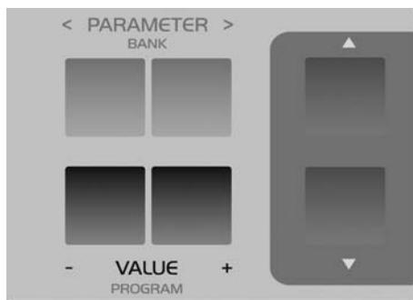
Use the UP or DOWN buttons to activate the filter section FILT. The second encoder knob in this row is labeled CUTOFF (not to be confused with CUTOFF 2!). Rotate the encoder to the left and right and note how the sound becomes muddier and clearer in response to the direction in which you turn the encoder. (To ensure this effect and the following aural experiments are
