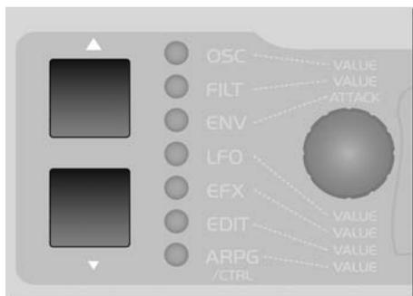
When you call up a parameter in the display menus, you will also be determining the function of the dedicated knobs (those with the fixed labels). If, for example, you select the LFO section, then the menu of one of the three LFOs is indicated in the upper line of the display. The parameter that is controlled via the VALUE knob
